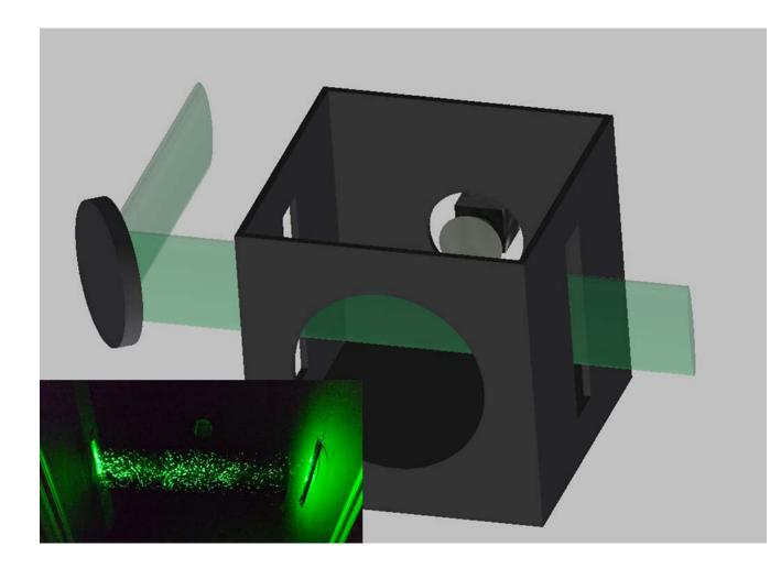
**Fig. 1. Schematic of the experimental setup.** A laser beam is expanded vertically by a cylindrical lens and shined through slits in the enclosure. The camera is located at the back of the box, a hole for the speaker in the front. The inset shows scattering for water particles from a spray bottle with the front of the box removed. Photo Credit: Martin Fischer, Duke University.
